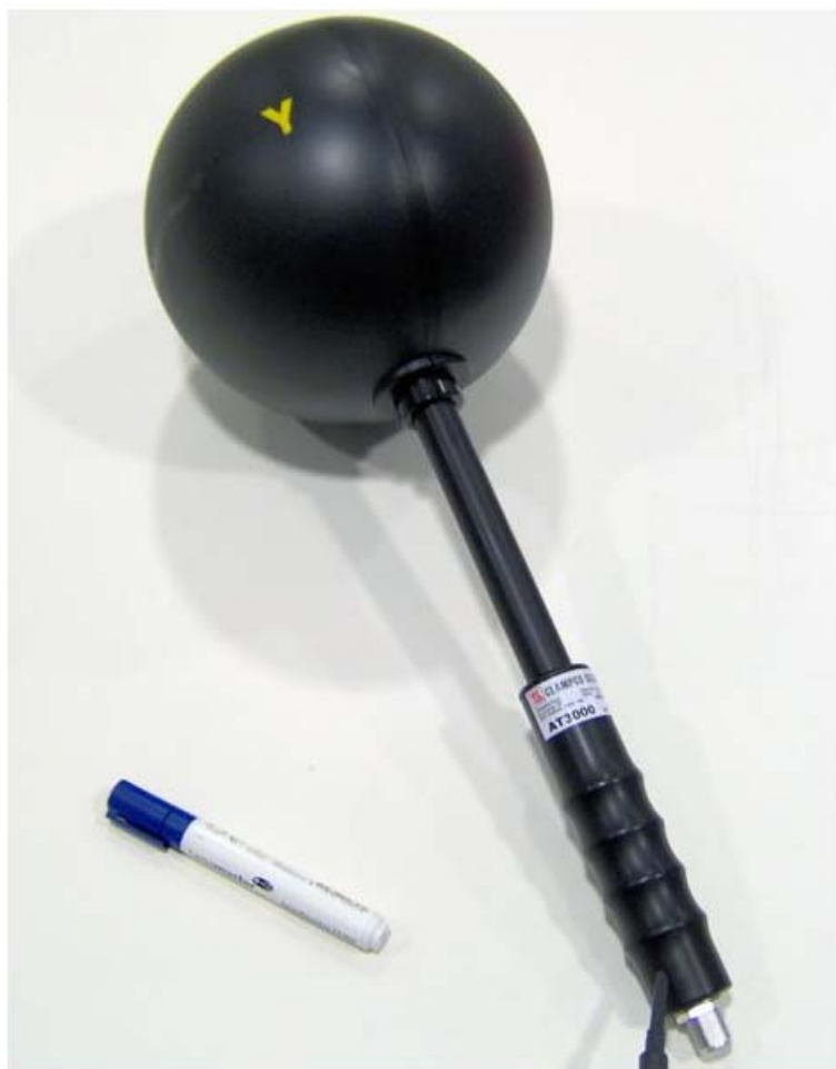
AT3000 is an isotropic antenna for EMF measurements in the range 20 MHz ÷ 3000 MHz
